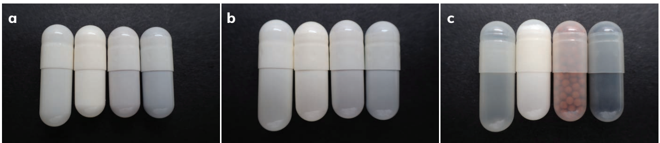
Figure 2b: Three sets of Hard gelatin capsules with different content. From left to right: (a) opacified with E171; (b) with alternative opacifying technology; (c) with calcium carbonate.
