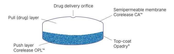
Combine with Corelease OPL™ a direct-to-hopper push layer designed for direct compression production of bilayer PPOP tablets.
