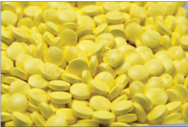
Appearance of tablets coated at 35 percent solids concentration
