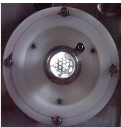
PhAT probe port view. Coater mesh is observed
