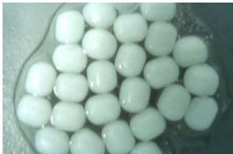
Figure 1. Appearance of the ER coated mini-tabs (10% WG) after 24-hour dissolution time
