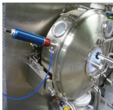
Coater Closed with PhAT probe in place looking into cascade
